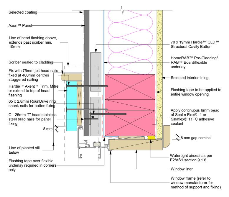
Note: When HomeRAB<sup>™</sup> Pre-Cladding/RAB<sup>™</sup> Board is used flashing tape to be applied to the entire window opening.
