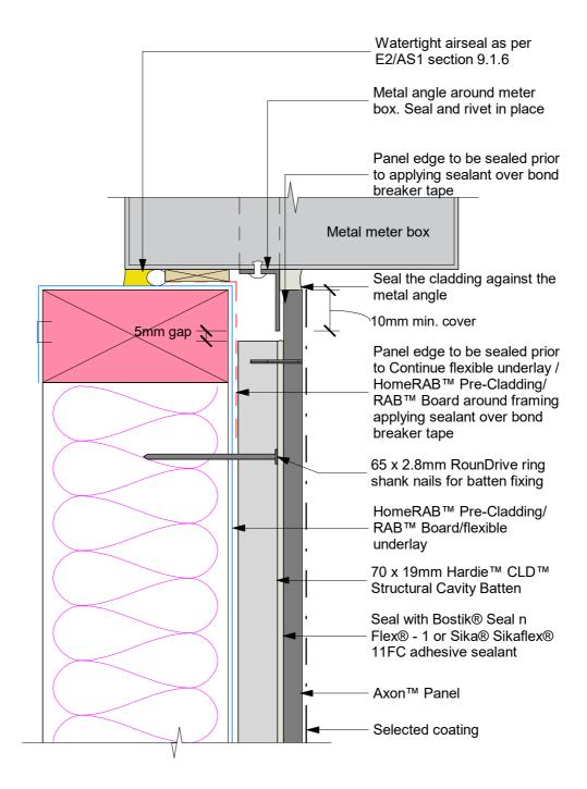
Note: When HomeRAB $^{TM}$  Pre-Cladding/ RAB $^{TM}$  Board is used flashing tape to be applied to the entire meterbox.
