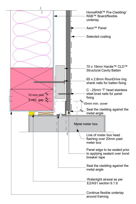
Note: When HomeRAB $^{\text{TM}}$  Pre-Cladding/ RAB $^{\text{TM}}$  Board is used flashing tape to be applied to the entire meterbox.
