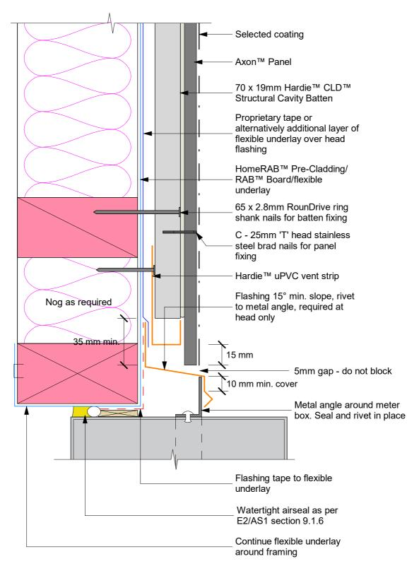
Note: When HomeRAB $^{\text{TM}}$  Pre-Cladding/ RAB $^{\text{TM}}$  Board is used flashing tape to be applied to the entire meterbox.
