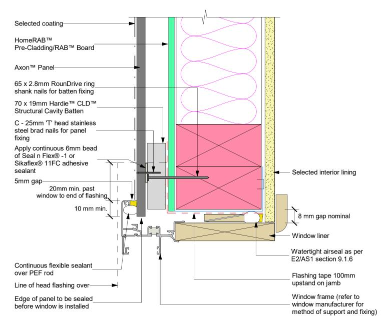
Note: When HomeRAB™ Pre-Cladding/RAB™ Board is used flashing tape to be applied to the entire window opening.
