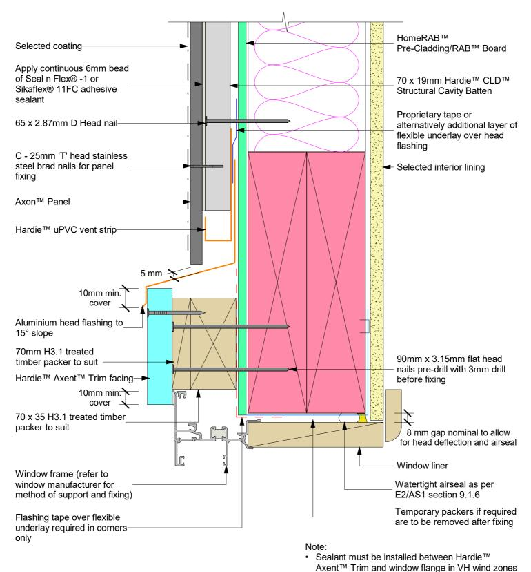
Sealant must be applied between the head flashing
