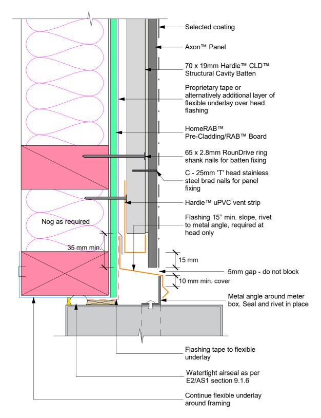
Note: When HomeRAB<sup>™</sup> Pre-Cladding/ RAB<sup>™</sup> Board is used flashing tape to be applied to the entire meterbox.
