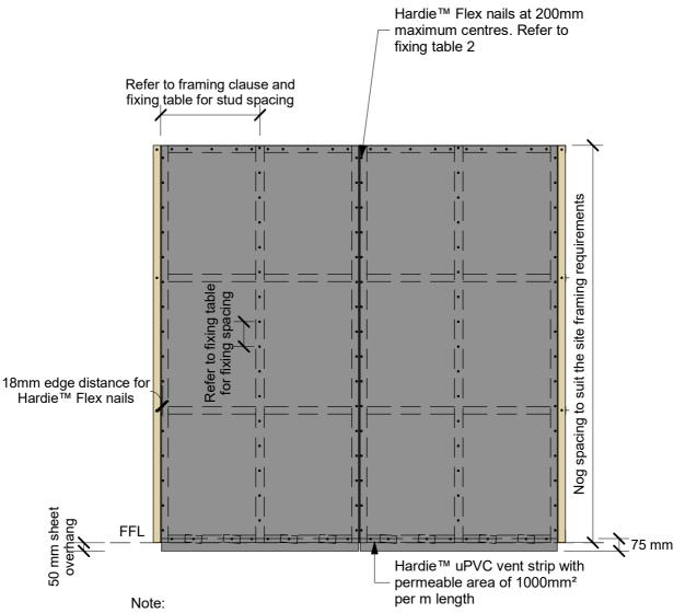
For fire rated wall systems by James Hardie nog spacing must be 800mm centres maximum
