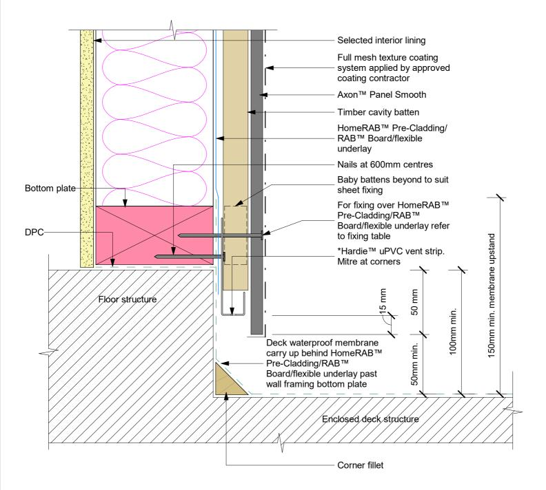
\*Drain holes in Hardie™ uPVC vent strip to achieve the required ventilation openings of 1000mm² per lineal metre
