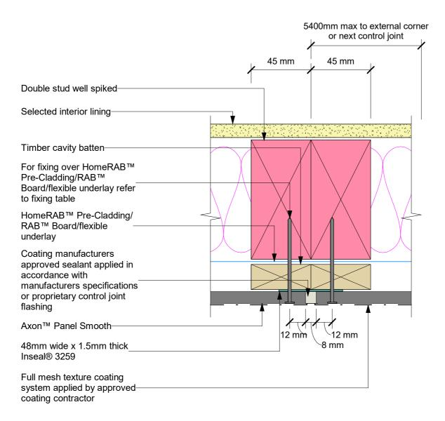
Edge of sheet to be sealed before sealant is applied, ensure compatibility with sealant. Note: Sealant must be colour matched to coating.
