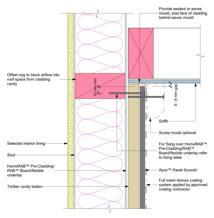
Note: Site cut edges to be primed. Ensure cavity does not vent into roof space. Refer to E2/AS1 clause 9.1.8.2
