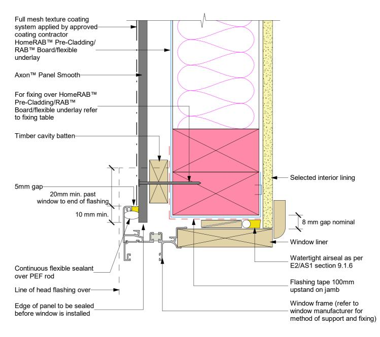
Note: When HomeRAB<sup>™</sup> Pre-Cladding/RAB<sup>™</sup> Board is used flashing tape to be applied to the entire window opening.
