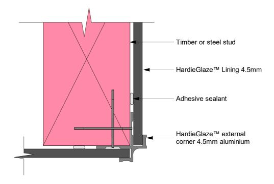
Note: For showers and similar wet areas the aluminium jointer must be silicone-sealant filled
