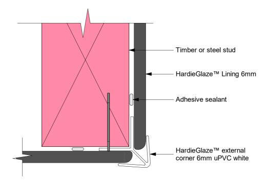
Note: For showers and similar wet areas the uPVC jointer must be silicone-sealant filled
