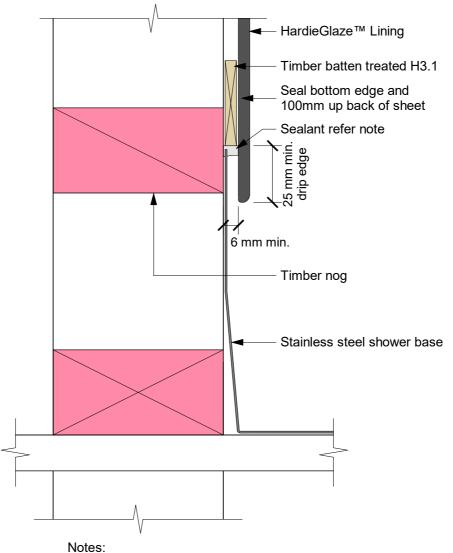
It is important to use sealant here to prevent possible damage to the framing.
