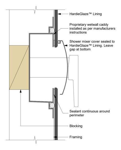
Note: Seal cut edges of HardieGlaze™ Lining
