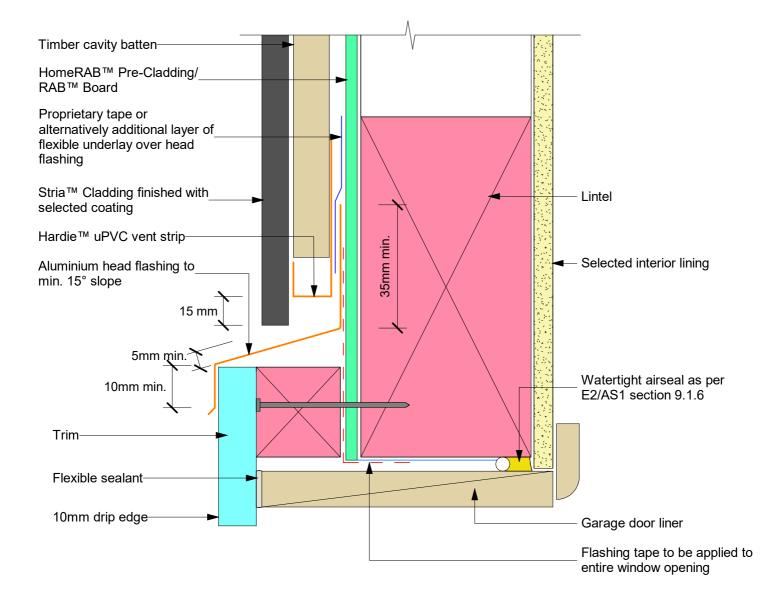
· Sealant must be applied between head flashing and Trim in VH and EH wind zones and SED wind pressures
