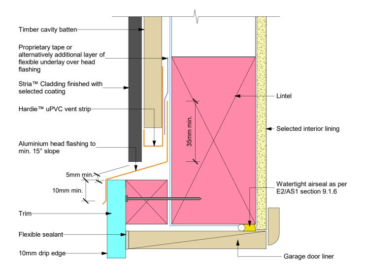
· Sealant must be applied between head flashing and Trim in VH wind zones
